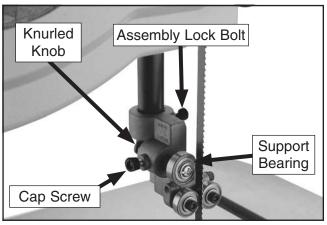
Figure 29. Upper support bearing assembly and controls.
